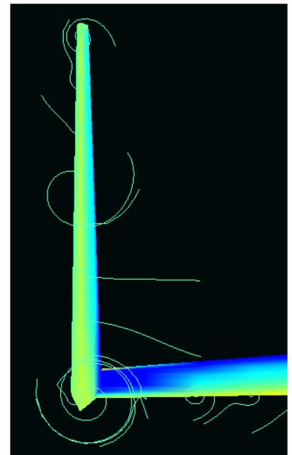
The next pair of pictures depict the same winglet with the leading edge aligned with the wing leading edge, similar to an **E-Racer** installation. Aerodynamicists claim this configuration has higher drag because the low pressure peaks on the wing and winglet coincide, leading to more mixing of the expanding air. Let's see what the analysis shows:
